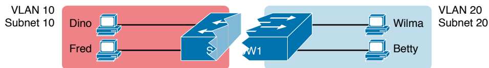
Figure 8-7 Layer 2 Switch Does Not Route Between the VLANs
