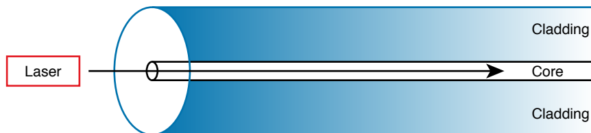
Figure 2-17 Transmission on Single-Mode Fiber with Laser Transmitter
