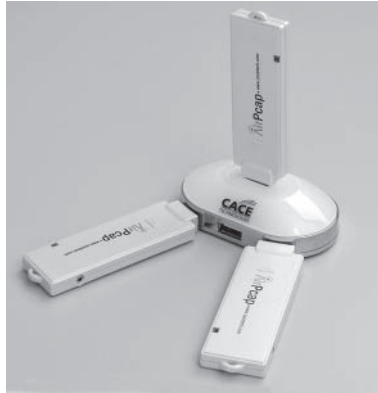
FIGURE 12.21 AirPcap provides multichannel monitoring and roaming analysis.
