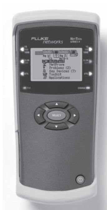
FIGURE 17.15 Fluke NetTool Series II inline network tester
