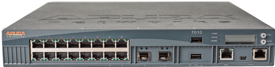
FIGURE 17.2 An Aruba 7010 wireless controller with PoE
